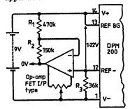
The voltage between Ref BG and Ref— is 1.22 V nominal. Resistors  $R_1$  and  $R_2$  should be low-drift types. The advantage of this circuit is that it avoids the temperature coefficient of  $D_5$  and the  $V_{bc}$  and  $H_{fo}$  coefficient of the BC212 transistor.
