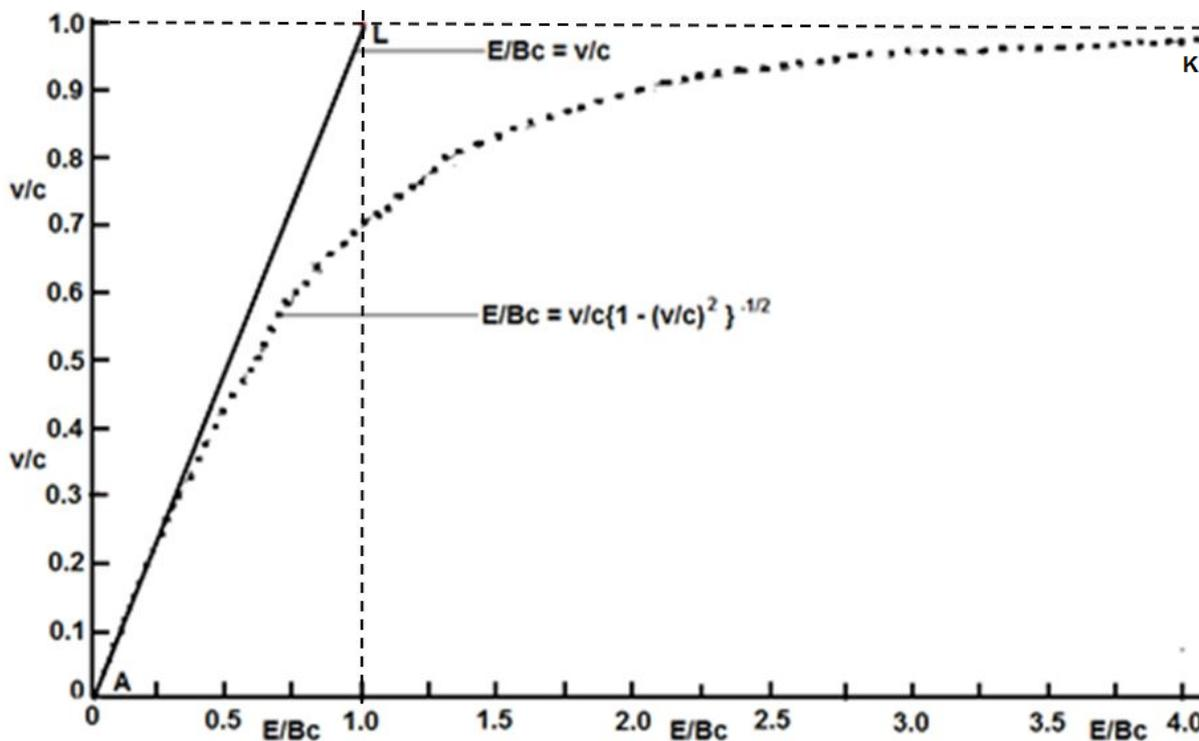
Figure 3. Graphs of speed  $v$ , in units of speed of light  $c$ , and electric field of magnitude  $E$ , in units of  $Bc$ , for a charged particle passing through a crossed electric field of intensity  $\mathbf{E}$  and a magnetic flux of intensity  $\mathbf{B}$ , at right angles, without deflection; the solid line  $AL$  according to classical and relativistic electrodynamics and the dotted curve  $AK$  according to an alternative electrodynamics.
