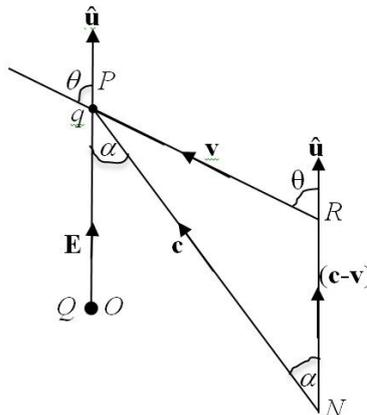
Figure 1. A particle of charge  $q$  at  $P$  moving with velocity  $\mathbf{v}$  at angle  $\theta$  to electric field  $\mathbf{E}$
