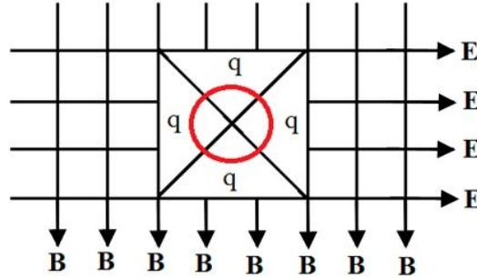
Figure 2. A particle of charge  $q$  passing with velocity  $v$ , perpendicularly into crossed electric field of intensity  $E$  and magnetic flux of intensity  $B$ .
