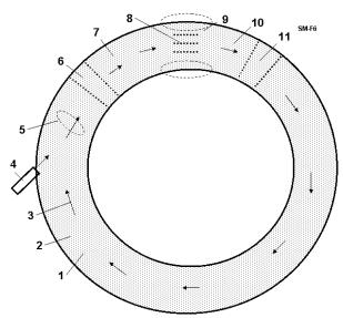
Fig. 12 Toroid producer of AB-needles (AB-matter). *Notations*: 1 – vacuum toroid; 2 – perpendicular (to sketch) magnetic lines; 3 – particles; 4 – particles gun; 5 – round magnetic lines from motion charged particles; 6 – electric accelerator; 7 – electric focuser; 8 – AB – needles; 9 – magnetic field keeping the AB-needles; 10 – electric focuser; 11 – electric accelerator.
