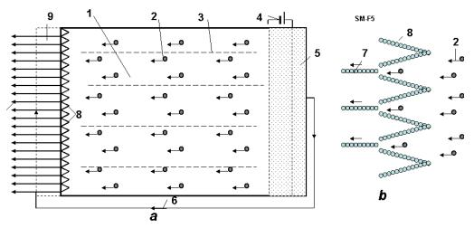
Fig. 13. Method particle traps for production of the AB-needles. *Notations*: a – device; b – particle traps; 1 - vacuum cell; 2- charged particles; 3 – magnetic lines; 4 – electric issue for the acceleration nets; 5 - plasma from particles; 6 – flow of electrons; 7 – AB-needles; 8 – trap made from AB-matter for the charged particles (p,  $^2$ H,  $^4$ He, etc.); 9 – cell for cover the AB-needles by electrons.
